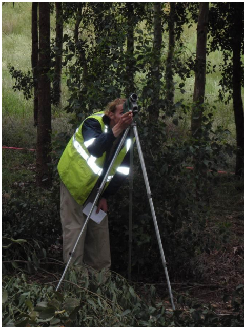
Mitch Haberkorn using a relascope to measure upper stem diameters in 8 year old E. bosistoana .
