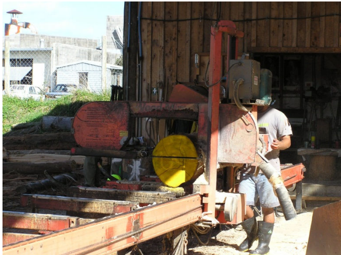
Figure 6: E. globoidea log being sawn, note lack of log movement as saw exits log
