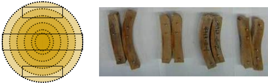
Figure 4. Four samples can be cut from each disc. Shrinkage is measured along their lengths, respectively in the radial and tangential directions.
