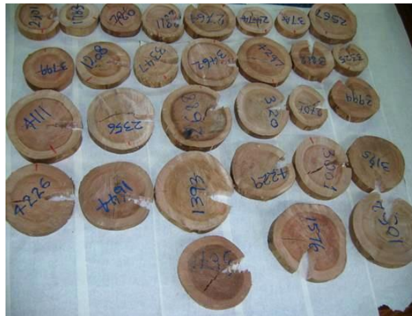
Figure 5. Differences in radial and tangential shrinkage can be assessed by leaving thin discs to dry.
