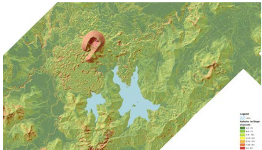
Slope data of an area in Northland taken by LIDAR. Photo: Landcare Research.
