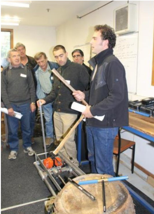
Figure 6: Dr Clemens Altaner, University of Canterbury's School of Forestry, describes the simple 'splitting' test for characterising growth stresses at the NZDFI workshop in Christchurch, 25 th May 2013.
