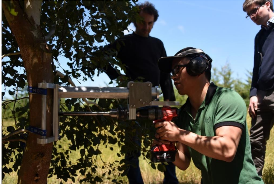
PhD student Yanjie Li tests the new coring tool on an E. bosistoana tree planted in 2009.
