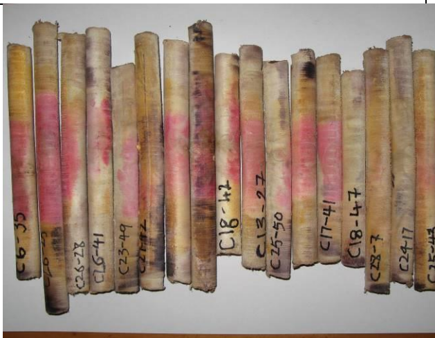
Cores stained with di methyl yellow that highlights heartwood by turning bright pink within minutes following application.
