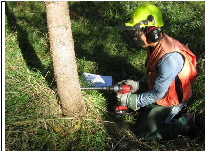
Corer used with a standard cordless drill.
