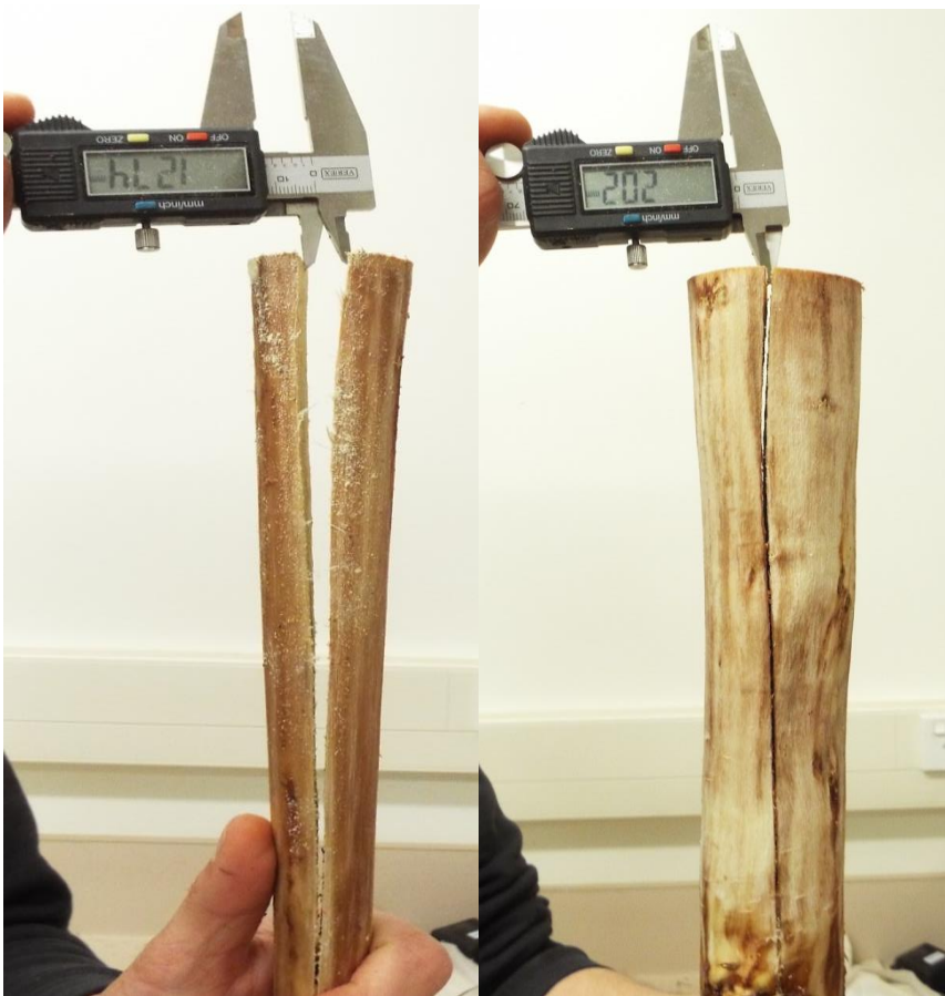
Figure 16: Measuring the opening (i.e. growth-strain) for 2 trees (step 7)
