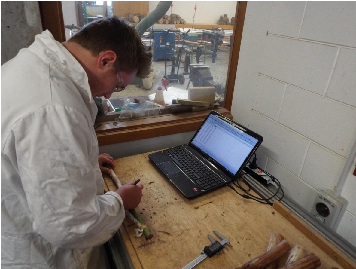
Figure 14: Measuring diameter and marking split length (steps 4 and 5)
