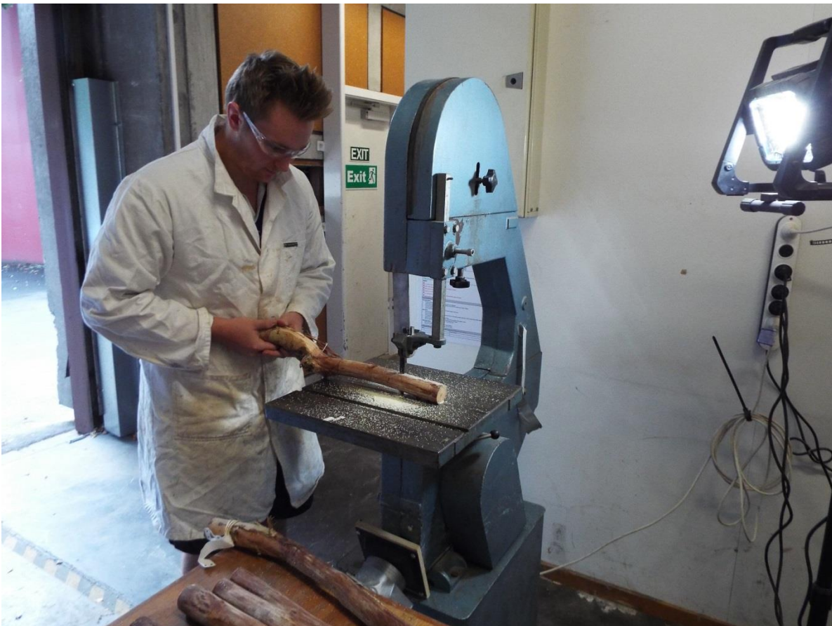
Figure 15: Splitting a sample (step 6)
