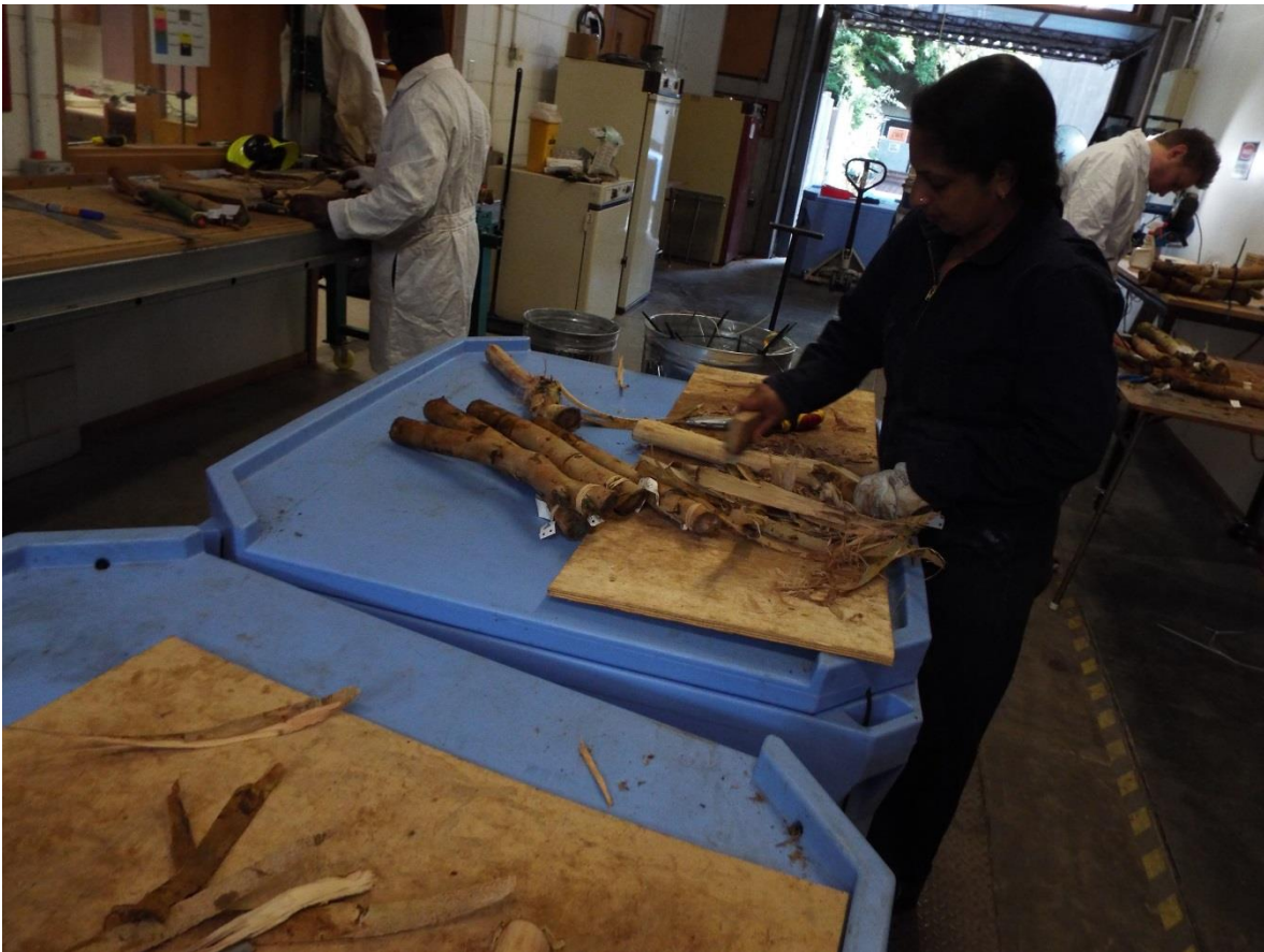
Figure 12: De-barking samples (step 2)
