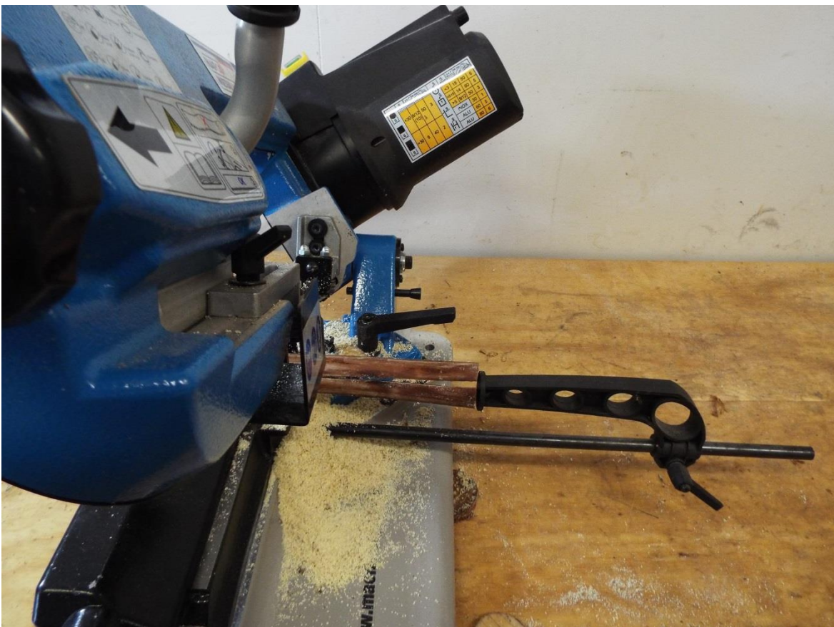
Figure 17: Docking samples for density, volumetric shrinkage and stiffness measurements (step 8)
