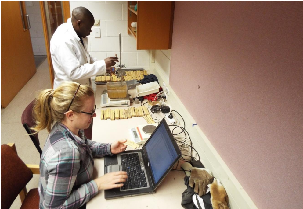
Figure 18: Measuring green mass and volume (steps 9 and 10)
