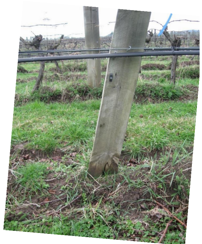
Figure 31: CCA treated pine post cracked across branch whorl at ground level and marked for replacement in vineyard 5.
