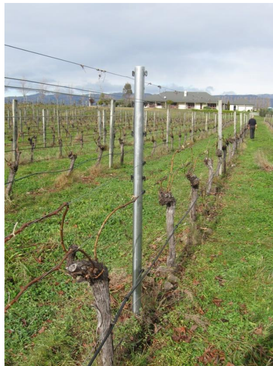
Figure 26: Eco trellis post manufactured by NZ Steel in vineyard 4a. This is a 1.15mm thick heavy zinc coated steel extruded to produce a 80 mm trellis post.
