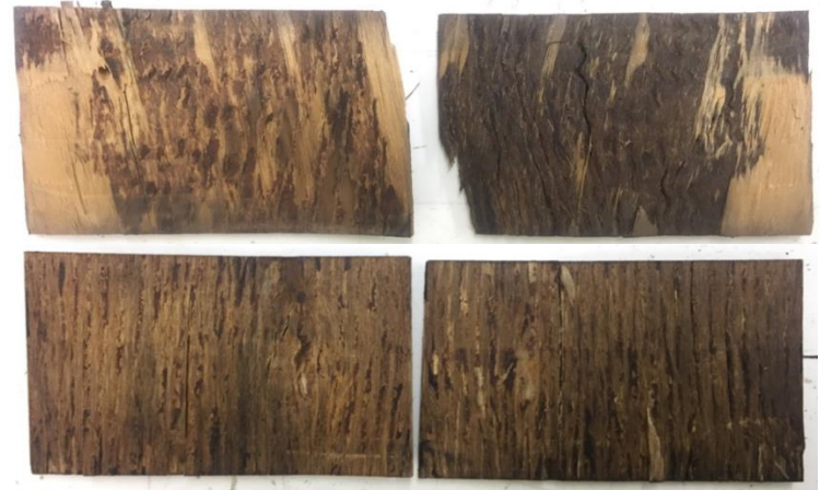
Gluelines with bond quality of 4 (top) and 0 (bottom)
