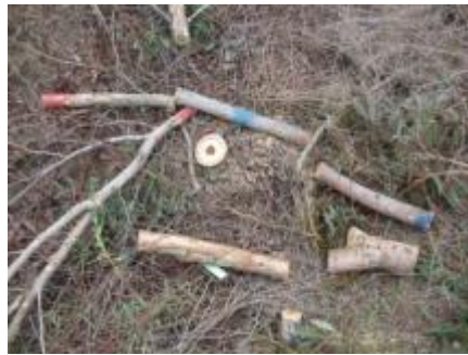
Figure 6: Harvesting stems for the splitting (growth strain) test (right).
