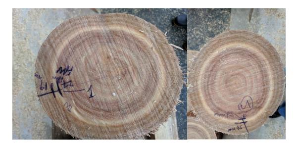
**Fig. 8.** Two typical cross-cut views of *E. globoidea* with the distinguishable sapwood, transitional, and heartwood zones.
