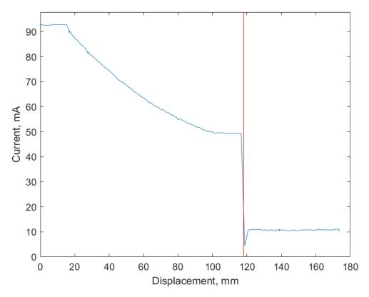
**Fig. 3.** Typical electrical current drop (blue) and switch position determined by the sapwood tool (red) in the tool verification test.
