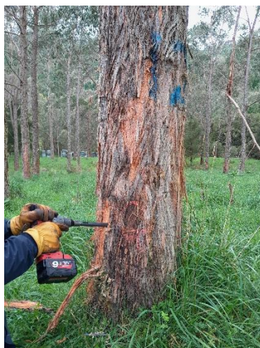
Figure 1. Coring an E. macrorhyncha tree using a battery-powered 14 mm diameter corer.
