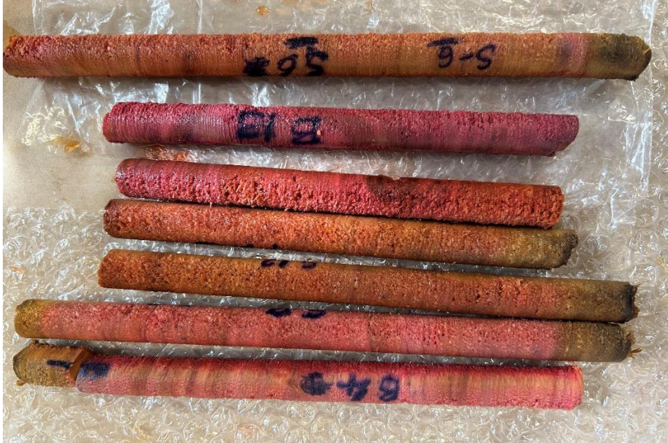
Figure 2. E. macrorhyncha cores with heartwood dyed pink after application of methyl orange.
