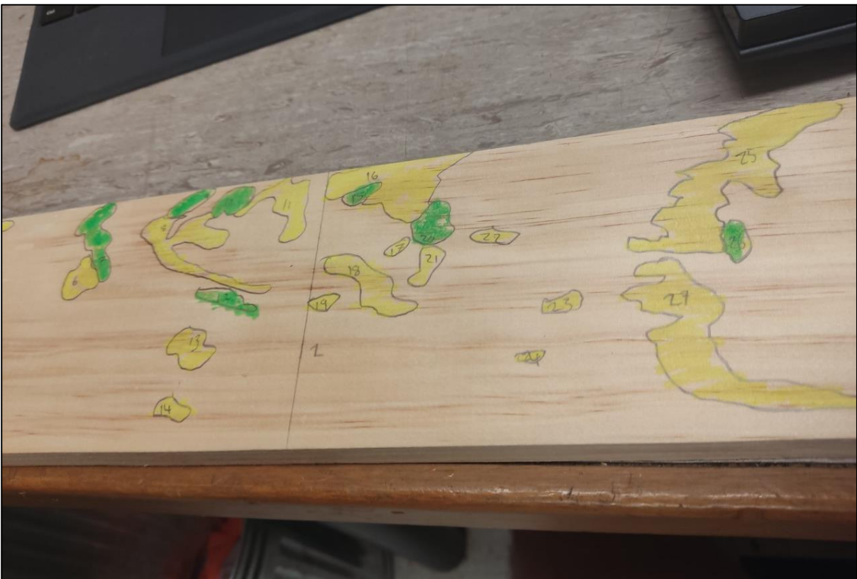
Figure 10: Example of coloured defects according to Table 4 on a Pinus radiata planed sample.
