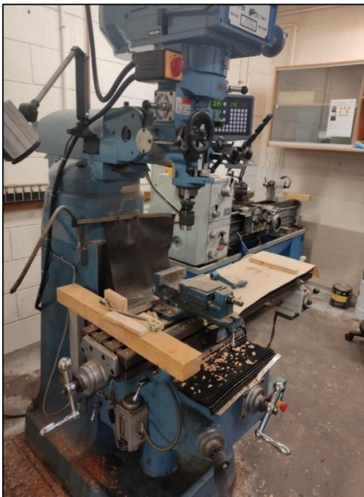
Figure 16: Luxcut TM-3VSL Turret Mill Used for Mortising.
