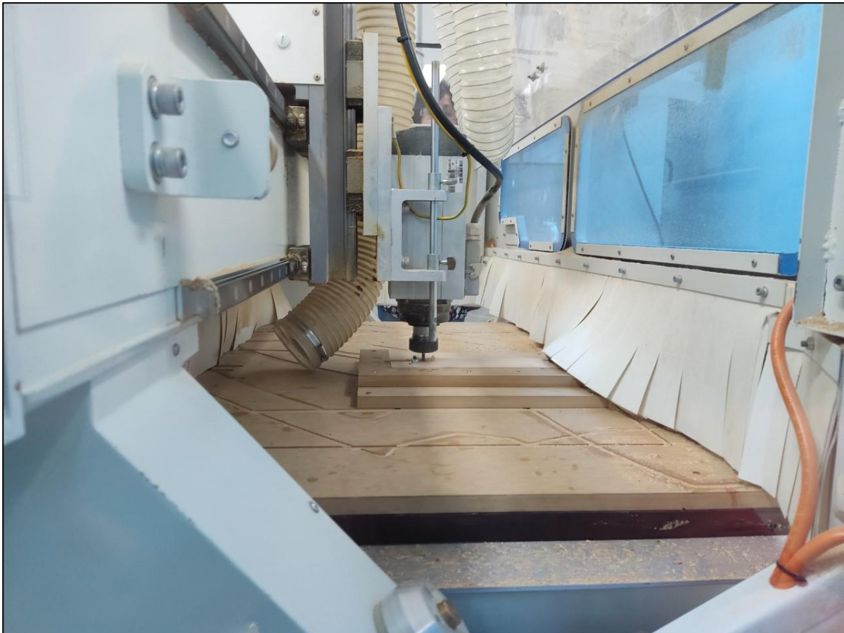
Figure 13: Ascent Pro CNC machine used for shaping.
