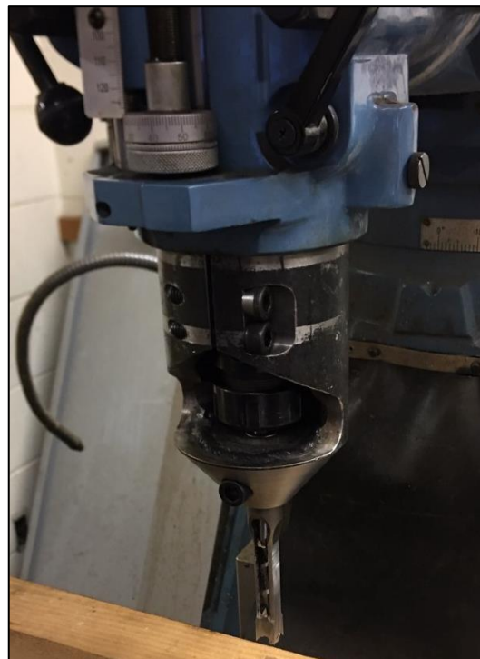
Figure 15: Custom Mortise Attachment for Turret Mill.
