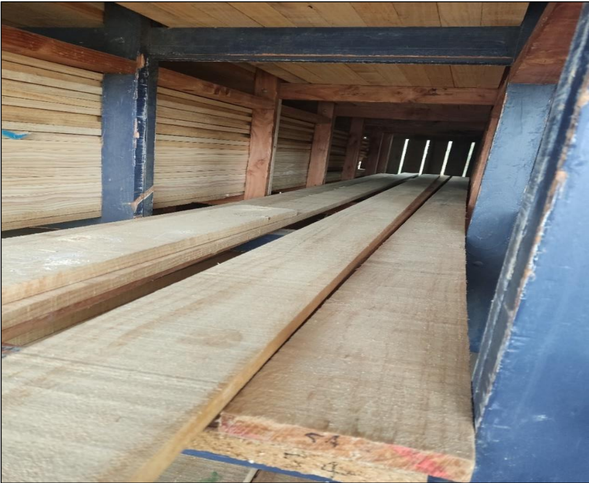
Figure 6: 5,200 mm x 150 mm x 25 mm kiln-dried rough, flat-sawn, Pinus radiata clears in stack at Halswell Timber. 2022.
