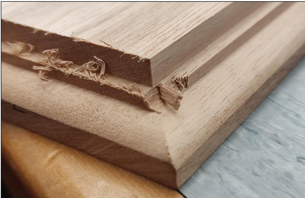
Figure 27: Example of typical defect on E. globoidea edge corner shaping.
