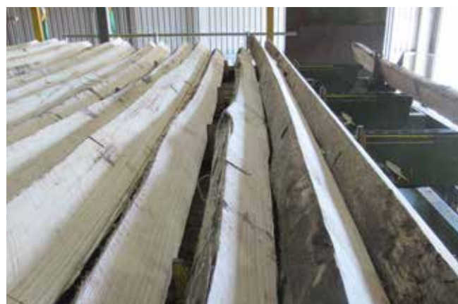
Radial sawn log sections at Radial Timbers mill in Yarram, south Gippsland
